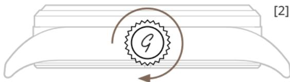
2. Wind the watch by turning the crown **CLOCKWISE** 20-55 times.
