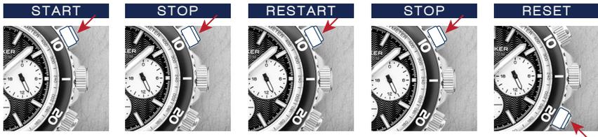
Restart and stop of the stopwatch can be repeated by pressing the button **A**.
