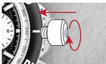
**TO SCREW:** Push the crown ALL THE WAY IN (towards the watch) THEN begin to turn clockwise until it is securely screwed down.
